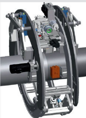
Figure 7: Automated laser beam welding with documentation of the weld test
